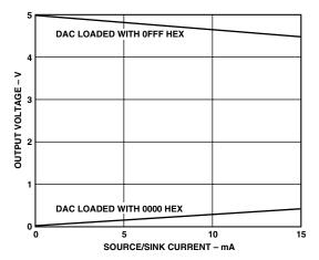
Figure 20. Source and Sink Current Capability with  $V_{REF} = V_{DD} = 5 \text{ V}$
